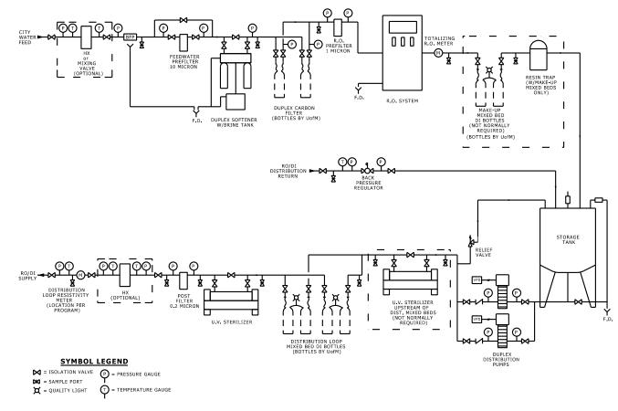
HIGH PURITY WATER SYSTEM SCHEMATIC
